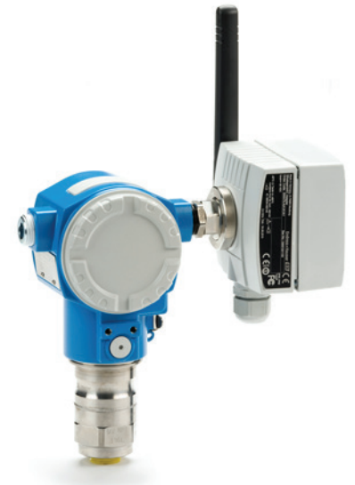
Example of an existing HART-enabled differential cell converted to a WirelessHART device by the use of the Fardux WirelessHART Interface FYI001.
