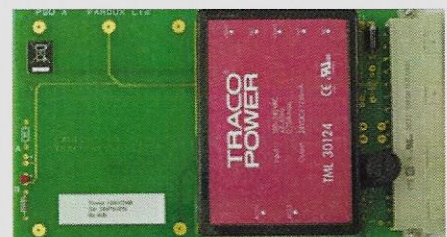
Figure 1: The power supply card fits into the backplane as shown in Figure 2.
