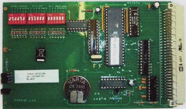
New 24 Bit Micro Processor card. (FDX/MIC/003)
