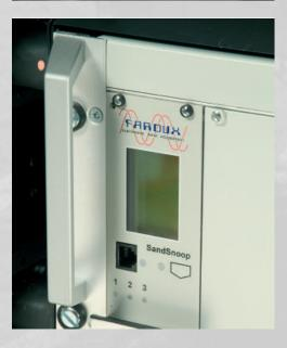
For produced sand or fracturing sand monitoring during flow backs the SandSnoop will measure and count sand impingements on the pipe wall and deliver this information in a variety of selectable units to the host software application.
