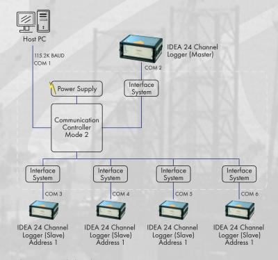
The Master and Slave loggers connect via the MLI to a single RS232 port
